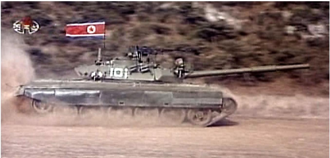
Vehicle #101. Note the missing front mud guard and the flexing side skirt panels. (Korean Central Television)
