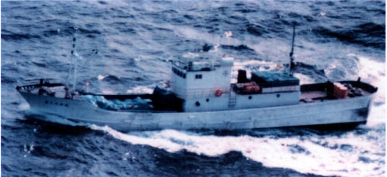
Views of one of the two DPRK infiltration vessels fleeing at high speed from JMSA and JMSDF vessels. Note how the specially designed hull allows the vessels to ride high and more easily slice through waves and swells. What appears to be the stern clam-shell doors to the internal “wet-well” are visible in the lower image. (Japan Maritime Self-Defense
