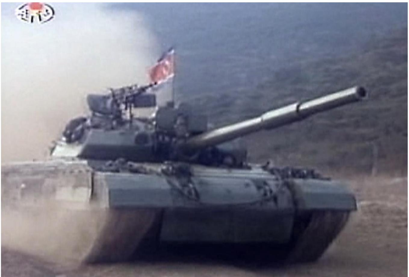
Vehicle #131. Note the tow cable on the glacis plate appliqué armor module and that the laser range-finder does not have a cover. (Korean Central Television)
