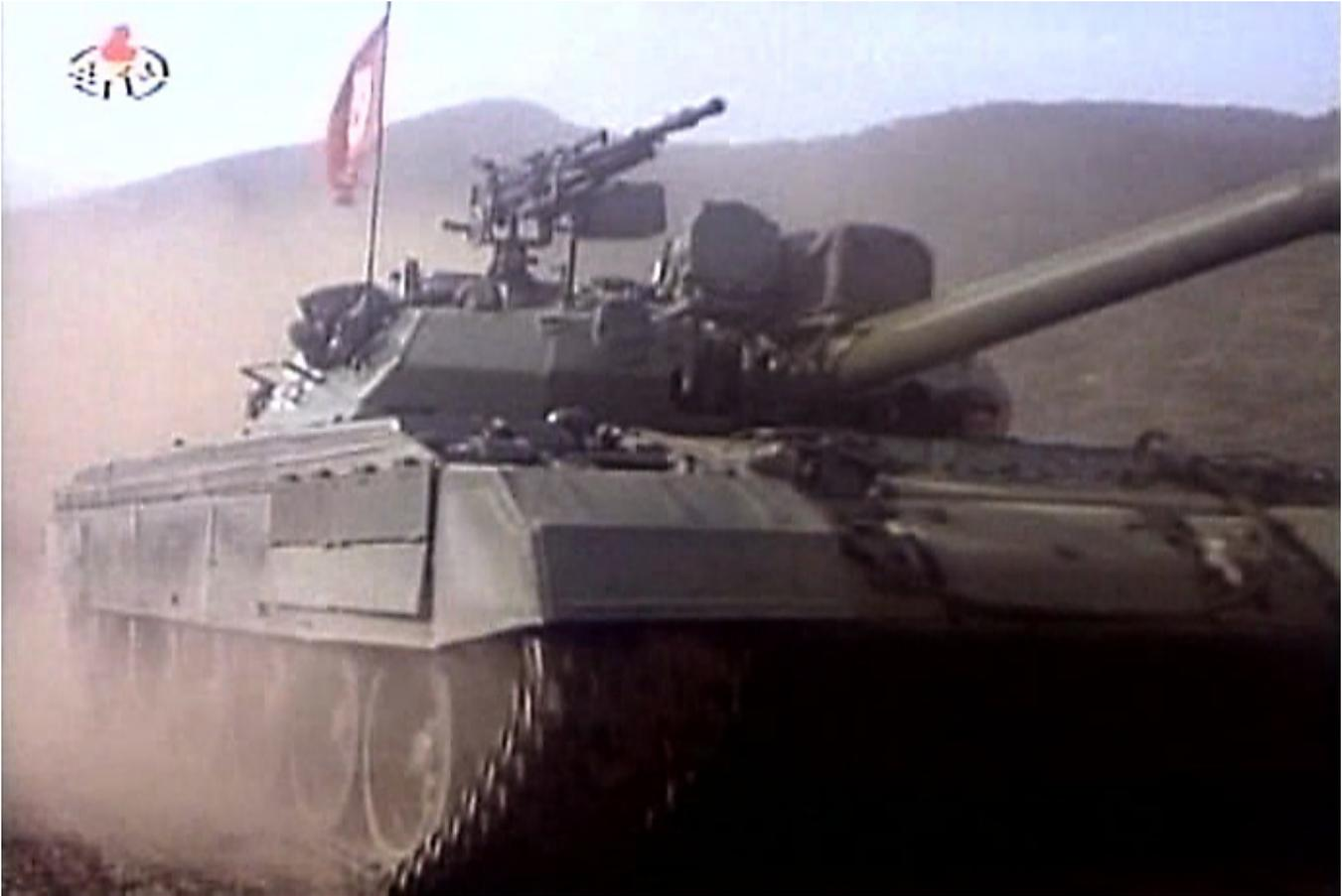
Vehicle #123. Visible in this image are the wedge-shaped laminate module on the front of the turret, glacis plate appliqué armor module, folding panels on the side skirt and laser range-finder (with cover) on the main gun. Note the driver on the left side of the tank as in the T-62. In the T-72 the driver sits in the center. (Korean Central Television)
