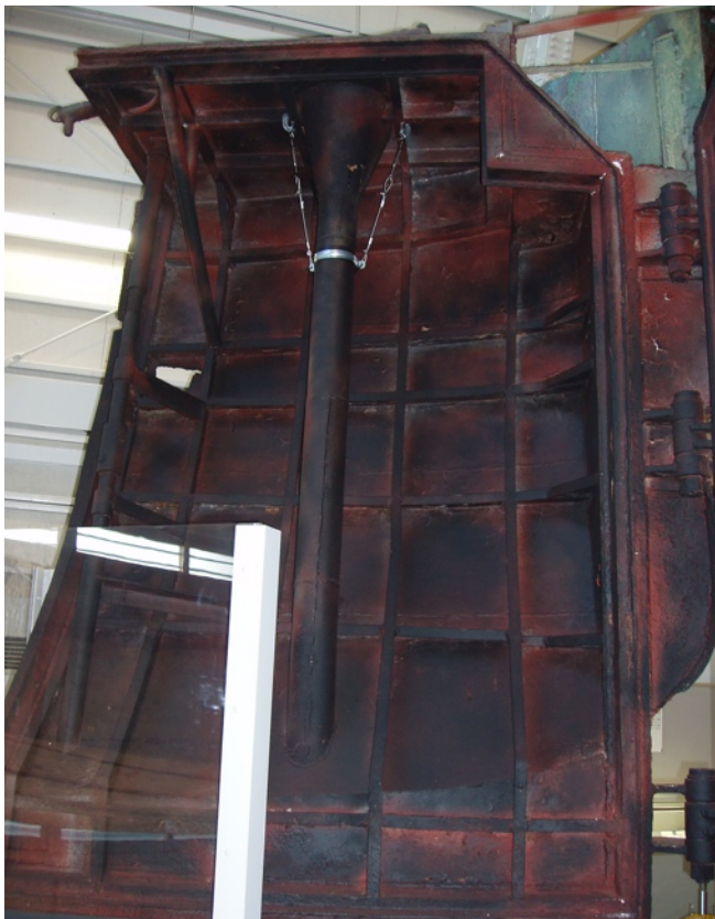
Details of the stern doors interiors. Note the gasket on the lip of the starboard door. (Joseph S. Bermudez Jr. collection)
