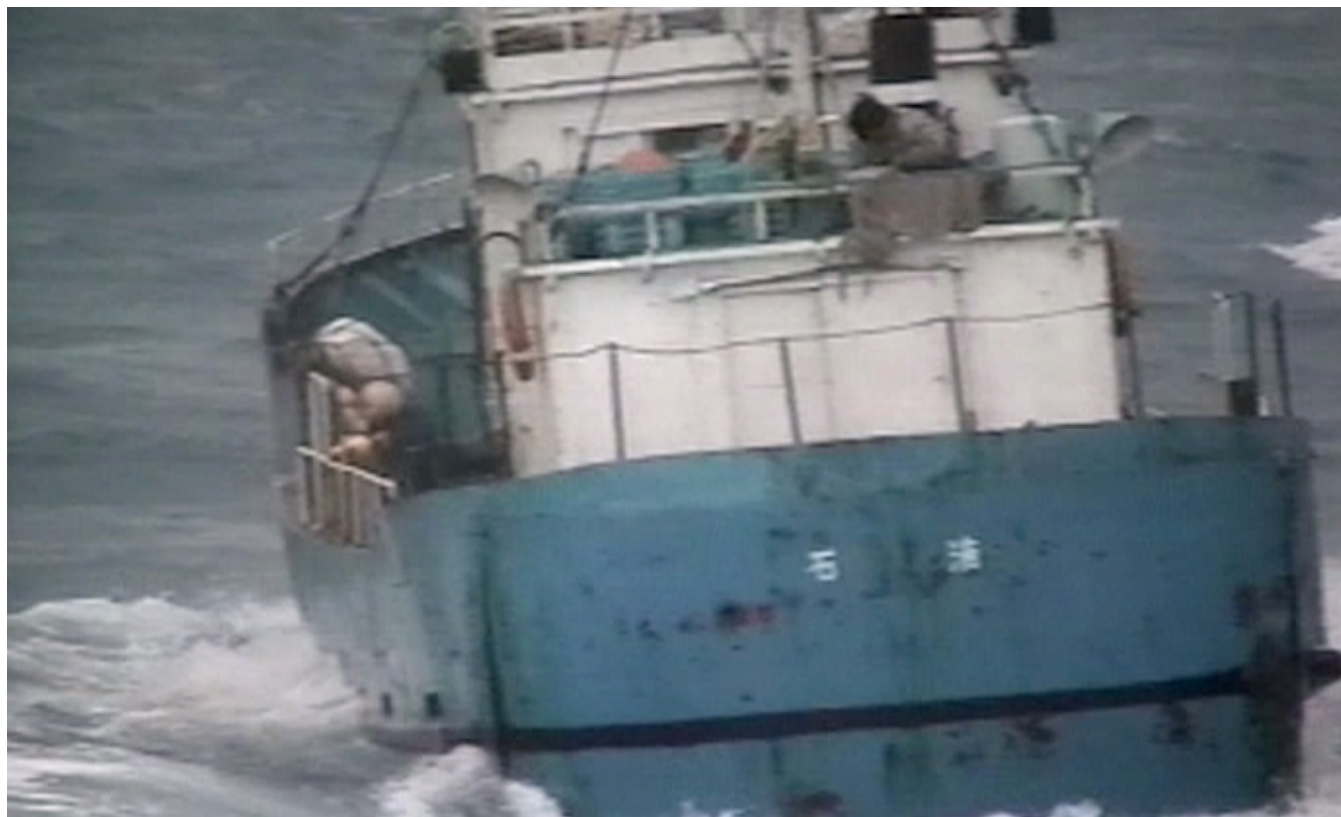
DPRK Infiltration vessel ("mother ship") attempting to escape from Japan Coast Guard vessels. The stern clamshell doors enclosing the "wet well" are just visible as vertical lines on either side of the hull. (Japan Coast Guard)
