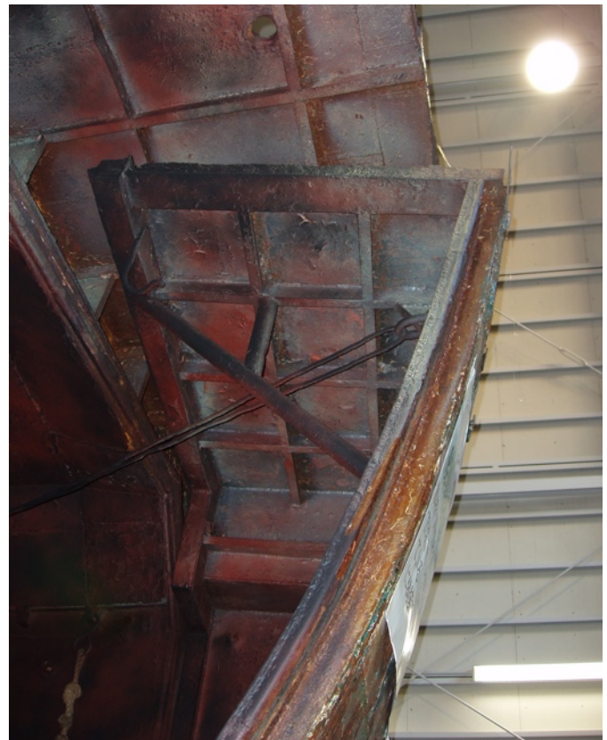
Details of the stern doors interiors. Note the gasket on the lip of the starboard door. (Joseph S. Bermudez Jr. collection)
