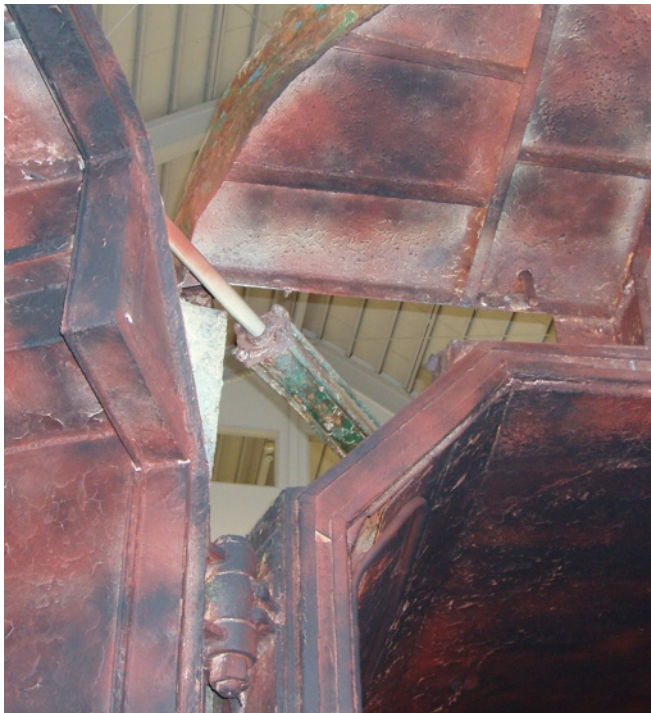
Detailed view of the upper hinge and hydraulic ram for the port door. (Joseph S. Bermudez Jr. collection)
