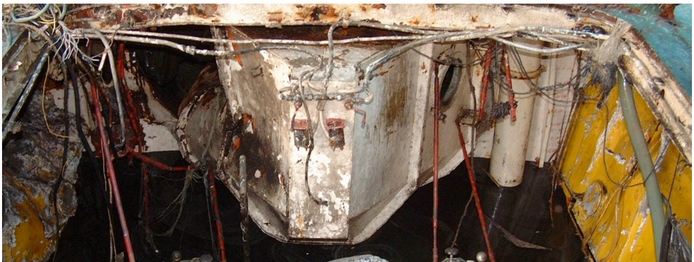
View of rear engine compartment looking aft at the extension to accommodate the ILC's bow. (Japan Coast Guard)
