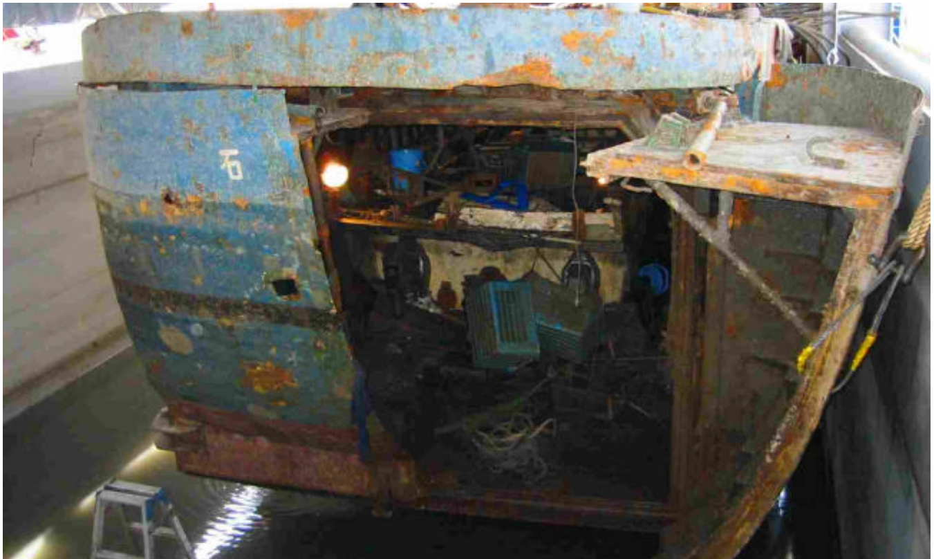
Stern view of infiltration vessel immediately after being salvaged. Note the high-speed infiltration landing craft (i.e., “daughter craft”) and debris inside the wet berth. (Japan Coast Guard)
