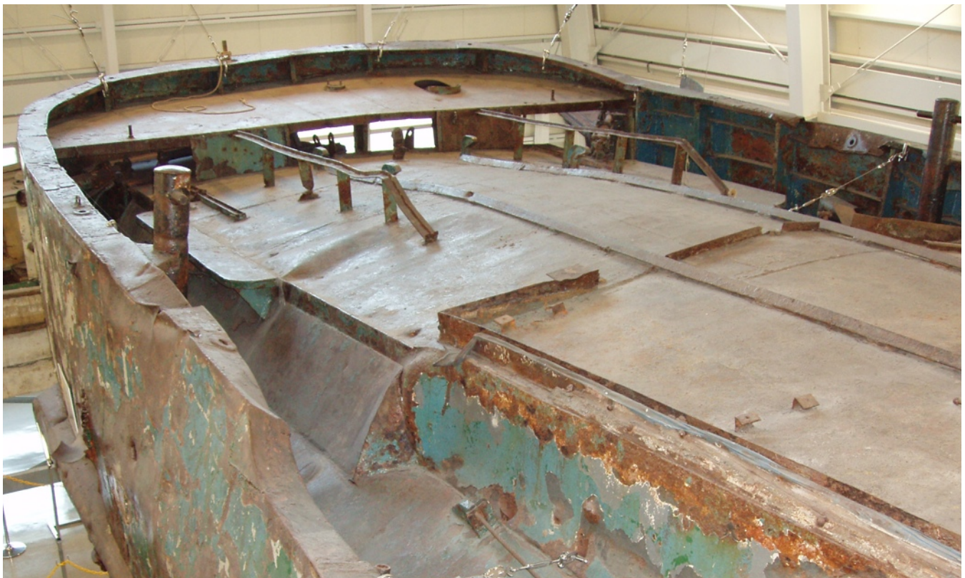
With the infiltration vessel now on permanent indoor display, a view looking aft showing details of the structure above the stern doors and how the deck was designed to provide the wet berth with head room. (Joseph S. Bermudez Jr. collection)
