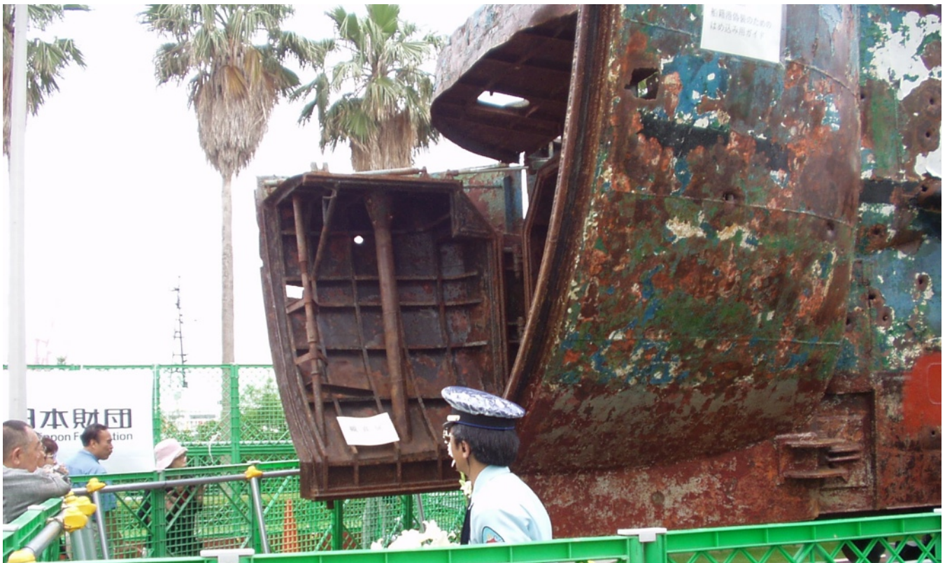
Now on temporary outside public display, this view shows the details of the clam shell doors. Not the hinges on the side of the hull, the hydraulic pistons and the gasket on the lip of the starboard door. (Ryoko Urakawa)
