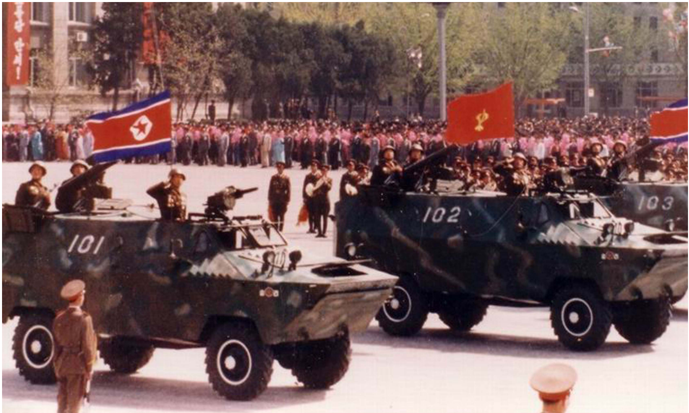
KPA M-1992/I AT-4 ATGM on parade in P'yongyang. Note the AGS-17 grenade launcher on the roof above the driver. (KCNA)
